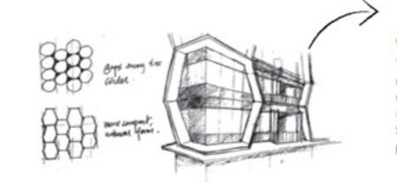
The facade is treated with bio-mimicry architecture inspired by nature. It is modelled after a beehive to provide shading from the sun and to create a unique and outstanding facade. This design philosophy is conceptualised in accordance to the stringent standards of the BCA Green Mark Platinum Standard, which is the nation's highest accolade for environmental design, performance and sustainability in property developments.
