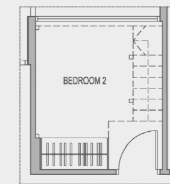
Suggested Furniture Loft (Only applicable to Bedroom 2 with maximum area of 5 sqm)
