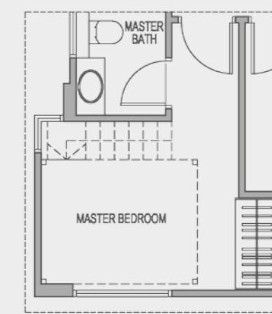
Suggested Furniture Loft (Only applicable to Master Bedroom with maximum area of 5 sqm)
